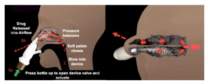
The drug delivery mechanism of the EDS is designed to overcome the drug deposition shortcomings of conventional nasal sprays and nasal aerosols. In conventional nasal sprays and nasal aerosols, the medication is inhaled or sniffed into the nose creating negative pressure within the nasal passages, which does not facilitate the
